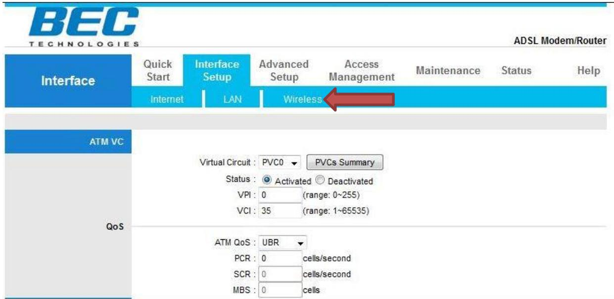
The screenshot shows the BEC Technologies ADSL Modem/Router web interface. The top navigation bar includes 'Interface', 'Quick Start', 'Interface Setup', 'Advanced Setup', 'Access Management', 'Maintenance', 'Status', and 'Help'. Under 'Interface Setup', there are sub-tabs for 'Internet', 'LAN', and 'Wireless', with a red arrow pointing to the 'Wireless' tab. The main content area is titled 'ATM VC' and 'QoS'. It contains the following settings:
